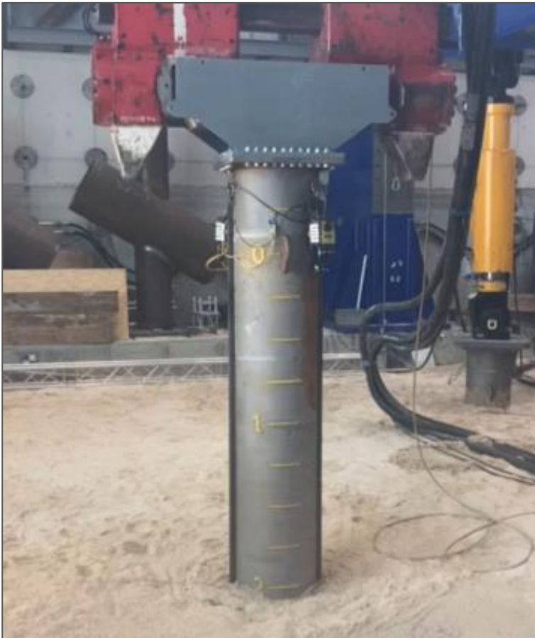
Able to successfully install with mesh via Vibrohammer
