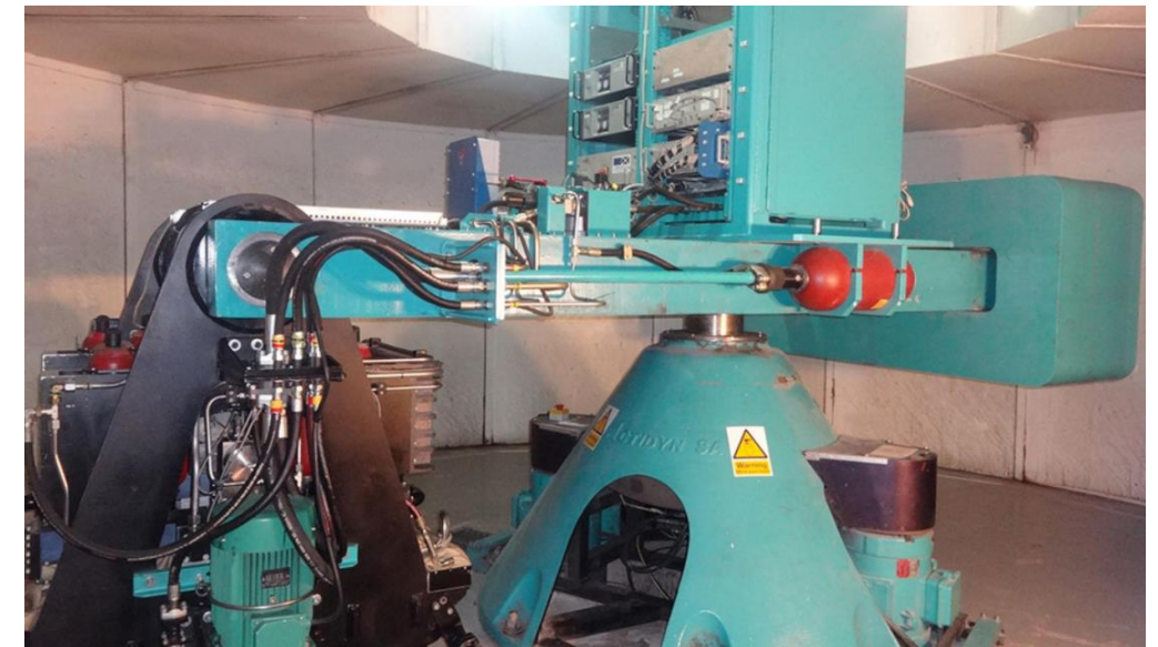
University of Dundee, Centrifuge testing of UMACK Anchors at 1:100 and 1:50 Scale
