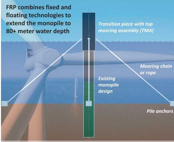
Patent Pending Fully Restrained Platform (FRP) Layout
