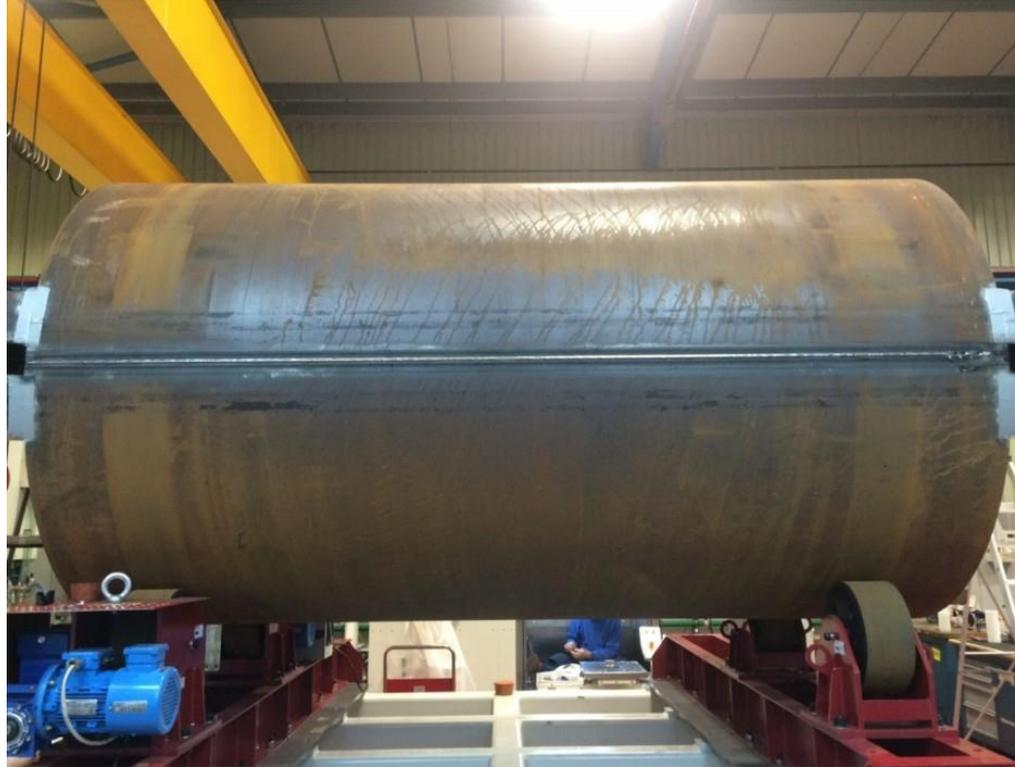
Commercialisation demonstration on 65mm 1.8m diameter S355 carbon steel.
