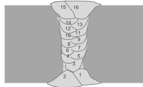
Schematic cross section of multipass Submerged Arc Weld
