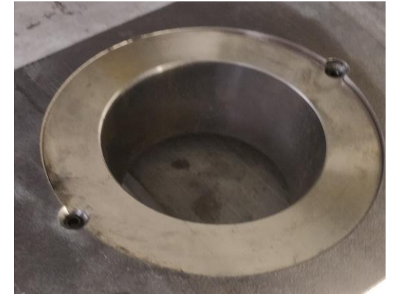
Repaired rotor lock
